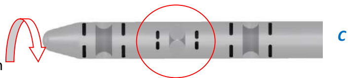
Incorrect Alignment of Markers for Distal Screws Insertion
