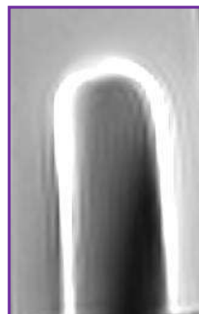
Titanium Rod Ø5mm in MRI field: demonstrates massive artifacts
